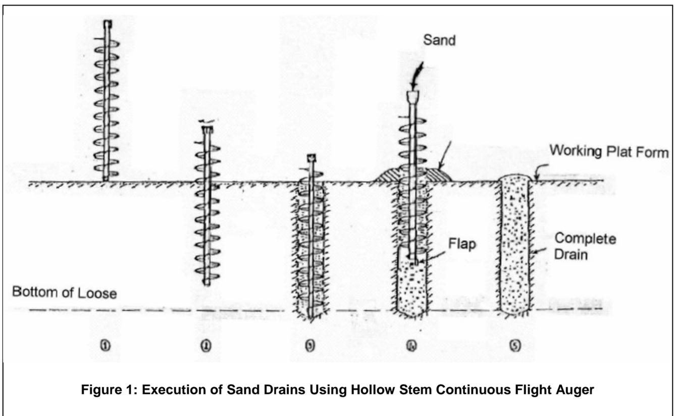
Figure 1: Execution of Sand Drains Using Hollow Stem Continuous Flight Auger
