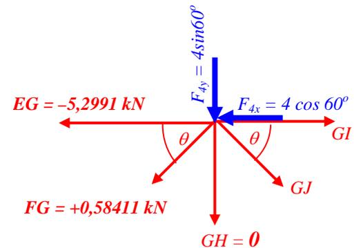
$$\Sigma F_y = 0 - 0,58411 \sin 53,13^\circ - 4 \sin 60^\circ + 0 + 0 - GJ \sin 53,13^\circ = 0 \Rightarrow \underline{\underline{GJ = -4,9142 \text{ kN}}}$$
