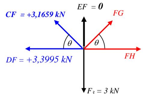
$$\Sigma F_y = 0 + 0 + 3,1659 \sin 53,13^\circ - 3 + FG \sin 53,13^\circ + 0 = 0 \Rightarrow \underline{FG = +0,58411 \text{ kN}}$$
