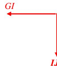
$$\Sigma F_x = -GI + 0 = 0 \Rightarrow \underline{\underline{GI = 0}}$$
